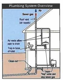
Drain pipes are designed as per Ontario Building Code to retain waterafter each use, in order to crea a water barrier that prevents odours from entering your home (see illustration to the right).
